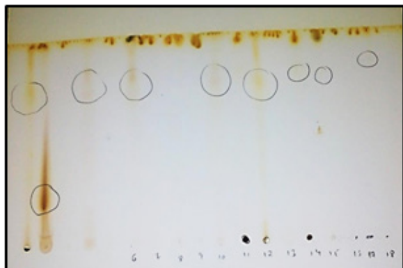
Fig-4. TLC Analysis. Some extracts showed distinct yellow spots (encircled) with Rf value 0.76, characteristic of saponins. The first lane from left is standard purified saponin, and the second lane from left is pure cholesterol.
