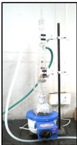
Fig-2. Setup of the Soxhlet Apparatus. The apparatus was set up in separate batches using methanol and petroleum ether as solvent. The yam sample (after coarse grinding) would be tied up using two layers of muslin cloth before being inserted into the siphon for the extraction process to occur. The temperature at which the extraction was carried out for each sample was determined by the respective boiling points of the solvent being used.
