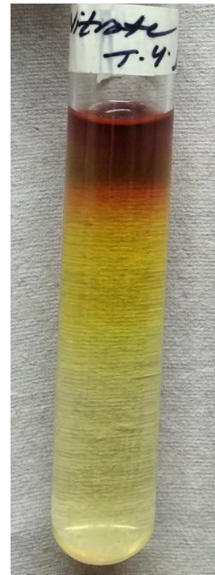
Figure 12: Formation of a red ring on addition of nitrate reagents indicates a +ve Nitratase Test.
