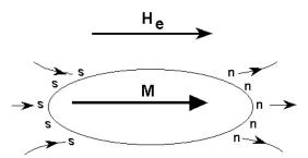
Magnetization Produces Apparent Suface Pole Distribution
