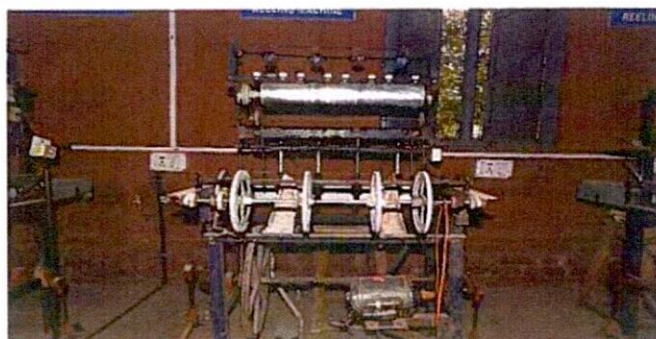
A reeling machine in the Sericulture unit of BAIF
