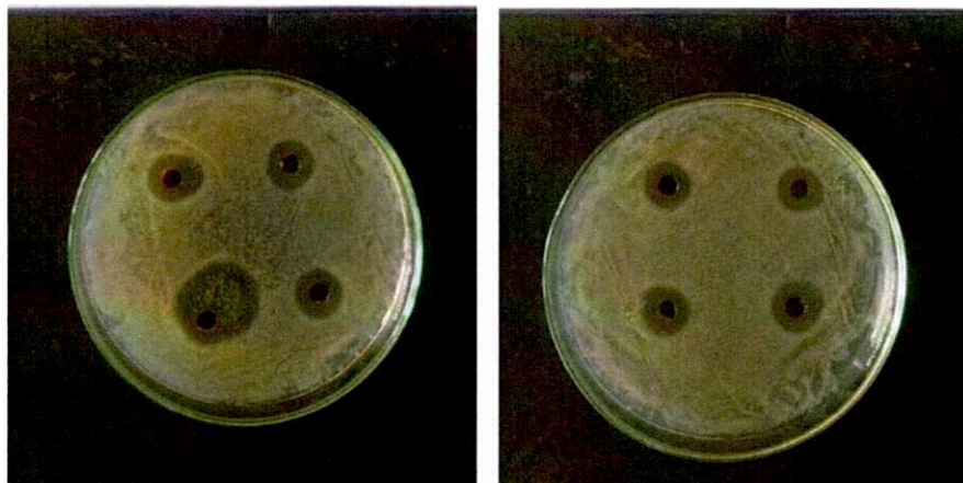
Figure 25: Zone of inhibition for 5mM Ag-NPs against E. coli (1mL of neem extract when added to 5mL of 5mM AgNO 3 )
